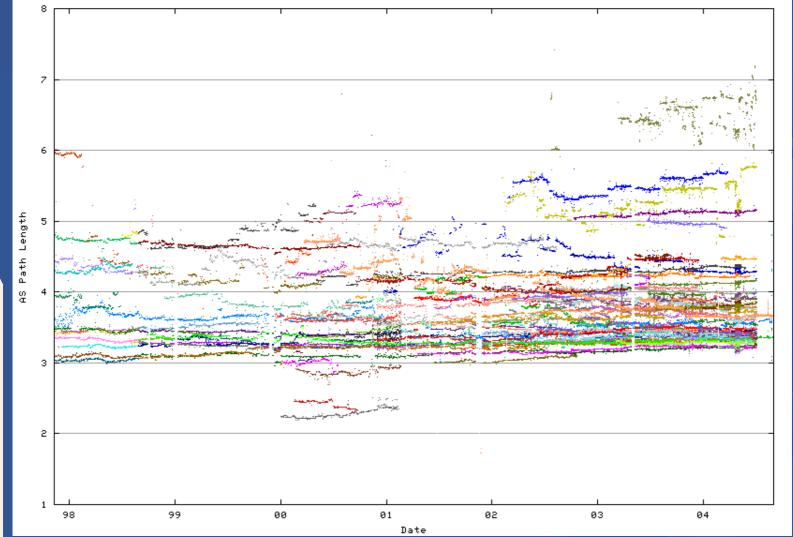
A constantly increasing number of ASNs can be related to average AS path length. The relatively constant AS path length for all AS paths implies that the density of AS increasing at a rate proportional to the number of ASNs being added.
