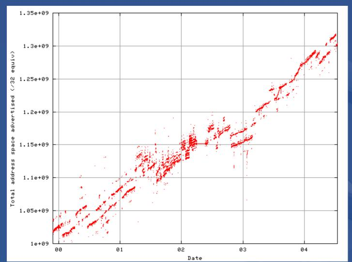
This is the same data for a single AS. It is evident thjast the number of unstable /8 advertisements has dropped from 3 to 1 over this period. It is also apparent that the rate of growth in 2004 is slightly higher than that of 2000.
