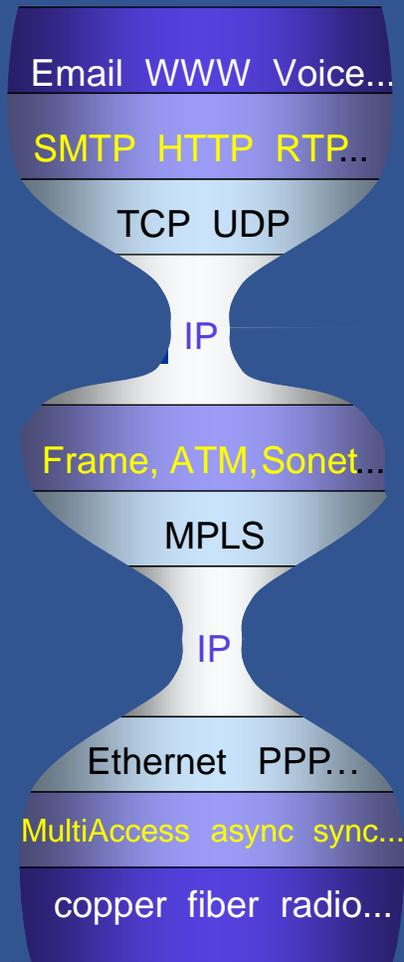
The addition of MPLS to the protocol model has caused some surprising outcomes in terms of using MPLS and IP as a substrate for emulated wire services
