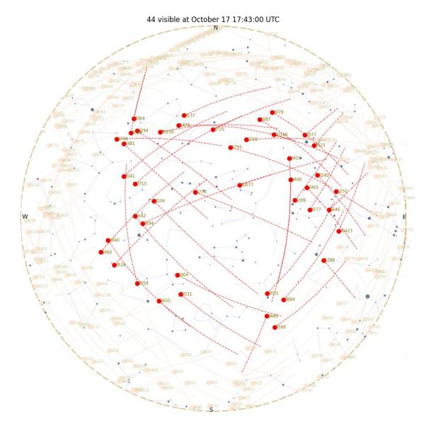
Starlink tracks satellites with a minimum elevation of 25°.
