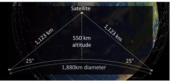
If you use a minimum angle of elevation of 25° then at an altitude of 550km each satellite spans a terrestrial footprint of no more than ~950Km radius, or 2M K<sup>2</sup>
