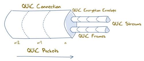
A QUIC connection is broken into "streams" which are reliable data flows — each stream performs stream-based loss recovery, congestion control, and relative stream scheduling for bandwidth allocation
